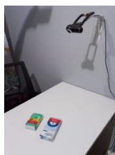
(ii) Webcam Setup 2 (45° angle between the optical axis and table plane, distance = 40cm)
